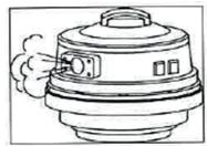
Push hose into blower port placed on the vacuum head. Turn the switch on.
